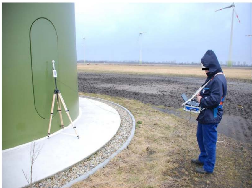
Fig. 3: Magnetic field measurement on E-101 (using a different sensor)
